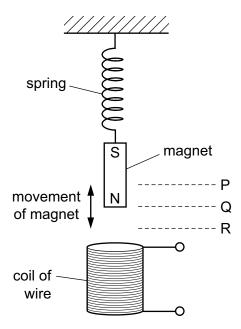
As the lower end of the magnet oscillates between P and R, a varying e.m.f. is induced across the coil.
