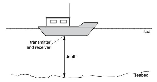
The depth of the sea beneath the ship is 600 m and the time measured is 0.80 s.
